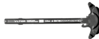
BCM GUNFIGHTER™ charging handle 556 • Handle machined from 7075 T6 billet • Hard coat anodized per Mil-A-8625F, type III, class 2 GFH BCM-GFH-556-MOD-A44: Ambidextrous BCM-GFH-556-MOD-4: Medium latch BCM-GFH-556-MOD-5: Small latch
