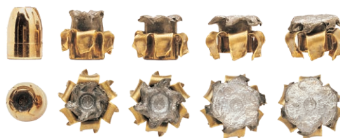
This series of photos shows the totally controlled and extremely uniform expansion of Golden Saber® HPJ bullets.
