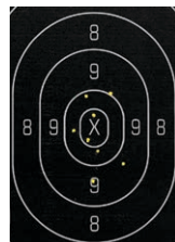
1 ROUND OF TAC 8 fired at 15 yards, IC Choke
